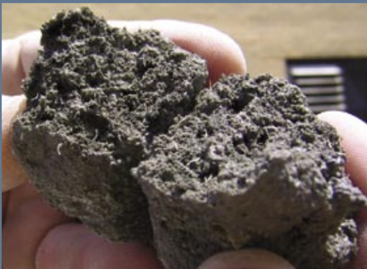
The very small UltraFiber 500® fibers can be seen protruding across the broken edge
