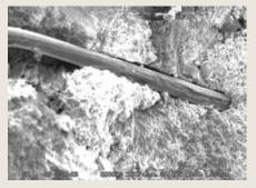
Fig. A: Note micro-voids around fiber and lack of paste/fiber bonding.
