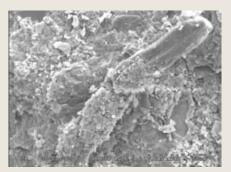
Fig. B: Cellulose fiber bonded into concrete.
