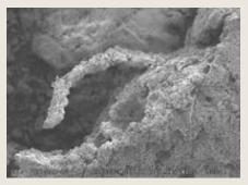
Fig. C: Cellulose fiber bonded with cement paste.
