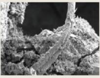
Fig. F: UltraFiber 500 in concrete after 4.5 years
